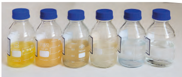
Figure 7: One set of samples from different points during a batch treatment. Left is the untreated wastewater and right is the completed effluent.
